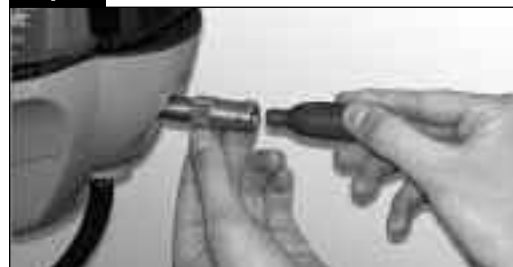
While holding the adapter in place, screw the Quick Clear cartridge into Quick Clear adapter.
