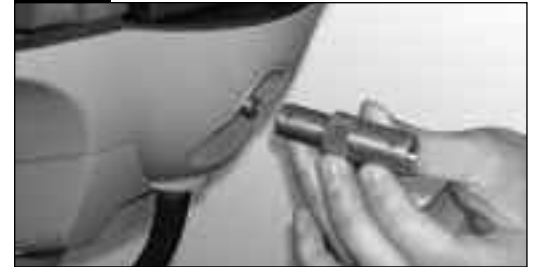
First hand-screw the Quick Clear adapter onto the valve.
